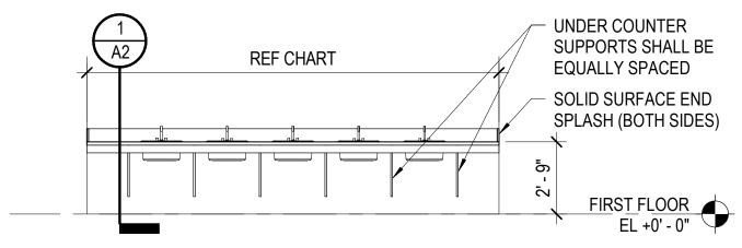
**NOTES:** SEE CHART FOR NUMBER OF SINKS AND UNDERCOUNTER SUPPORTS. COORDINATE FINAL SINK LOCATIONS WITH EXISTING PLUMBING ROUGH-INS.
